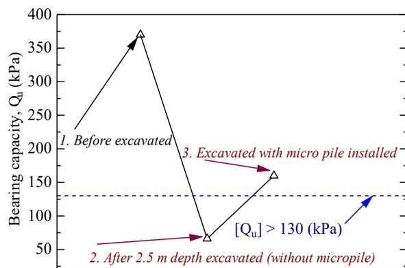
Figure 5. Effect of excavation and micropile installation on bearing capacity.
