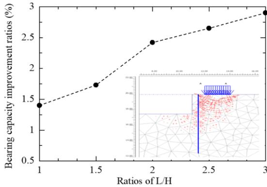
Figure 8. Effect of pile length on BCR.
