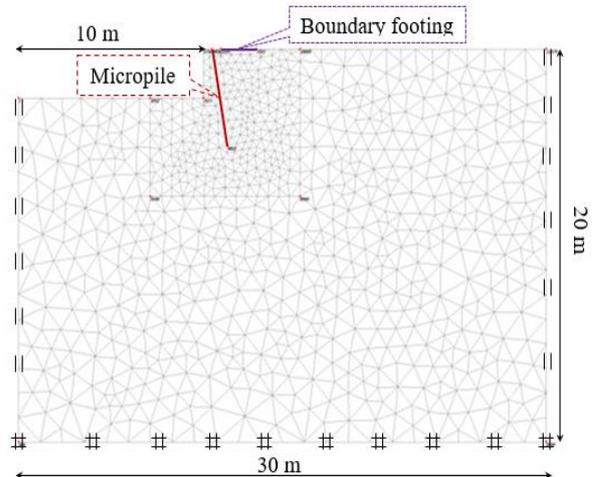
Figure 4. Geometry model, mesh generation, and boundary conditions.
