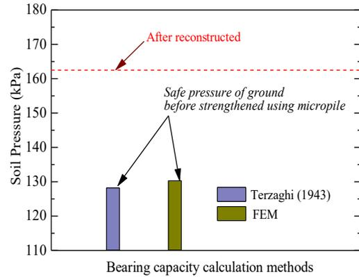
Figure 1. Soil pressure under the boundary footing before and after reconstructed.
