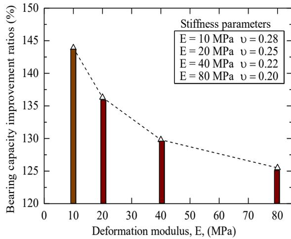
Figure 11. Effect of stiffness parameters on BCR.
