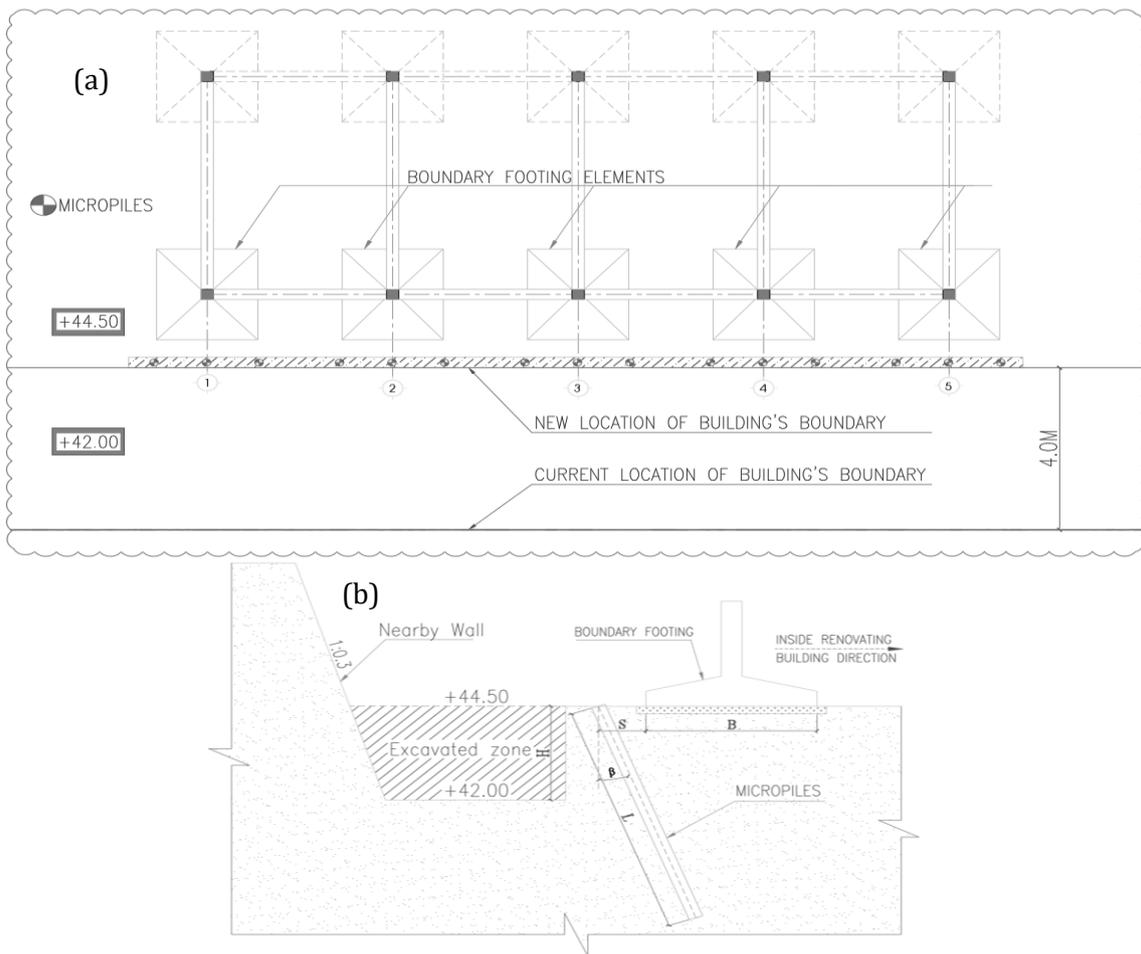
Figure 2. (a) Layout plan of foundation; (b) Cross-section of boundary footing after strengthened.
