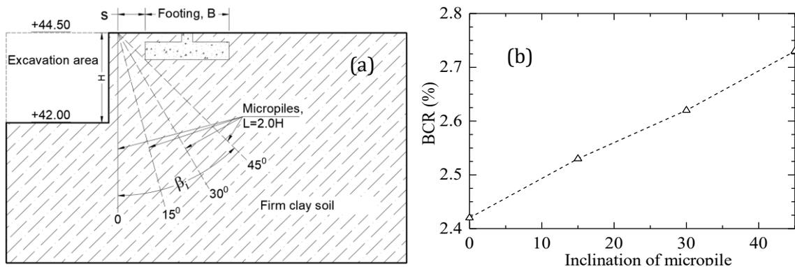
Figure 7. Effect of pile slopes on BCR.
