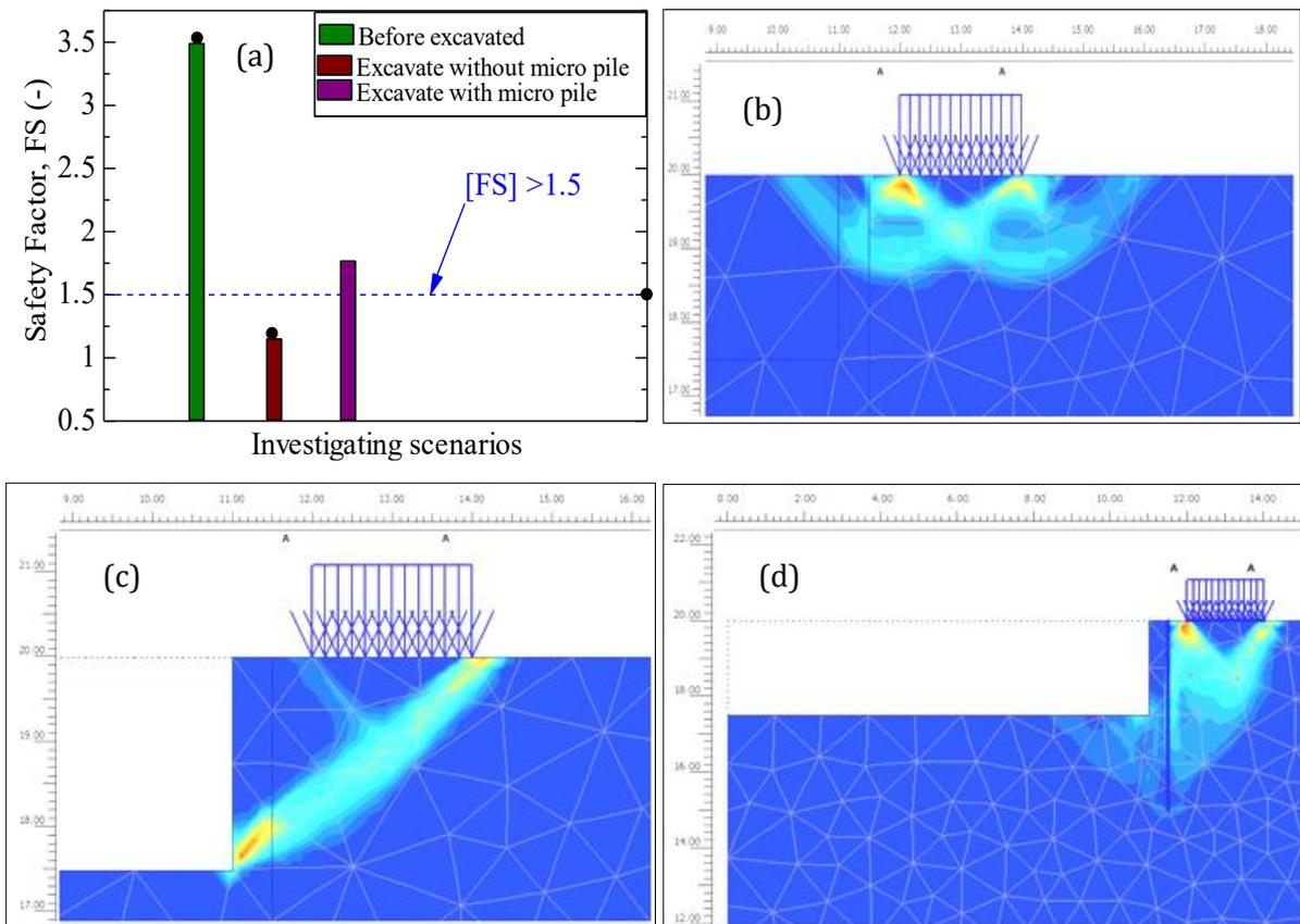
Figure 9. Stability analysis result of the foundation below the boundary footing.
